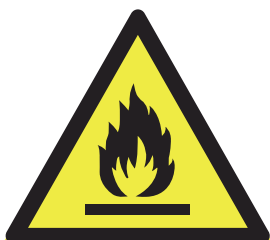
Caution: Risk of fire/ flammable materials
